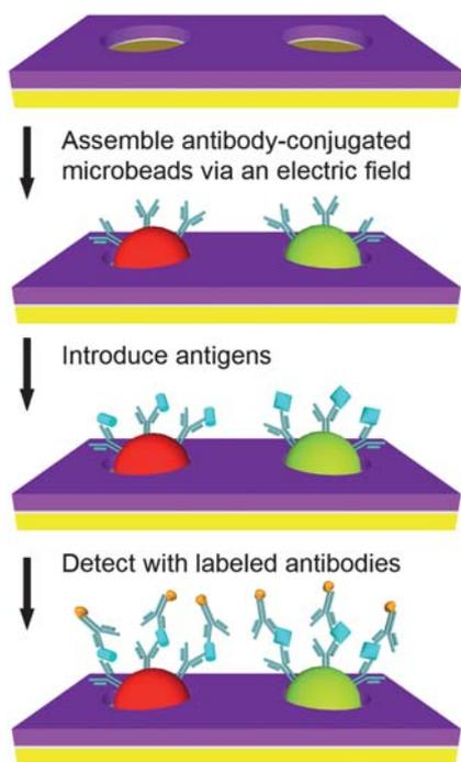
**Fig. 3** Sandwich immunoassay on antibody-conjugated microbeads assembled *via* electrophoretic deposition. Antibody-conjugated microbeads are assembled on the microfabricated arrays *via* the application of a pulsed electric field. Multiplexed protein detection is then performed within the same microfluidic channel using a sandwich immunoassay. Drawings are not to scale.
