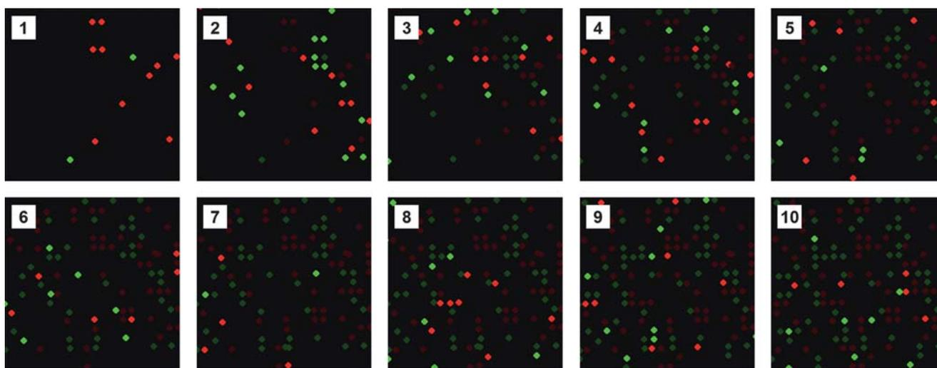
**Fig. 5** Spatial and fluorescence encoding of antibody-conjugated microbead arrays. Fluorescent micrographs of a small portion of an antibody-conjugated microbead array assembled in a stepwise fashion over the course of ten rounds using two different fluorescent microbeads (Panels 1–10). In panels 2–10, the brightness of the previously assembled microbeads has been reduced to emphasize the newly assembled microbeads.
