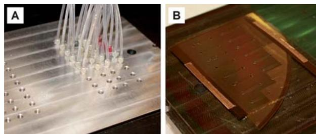
**Fig. 2** Photographs of the assembled electrophoretic fluidic device. (A) Top view of the custom-built aluminium plate through which the fluidic connections are made to each channel in the device. (B) Bottom view of the plate and an assembled device containing 14 separate channels. The bottom side of the aluminium plate has been coated with titanium and silicon dioxide films to aid in the adhesion of the double-coated tape.
