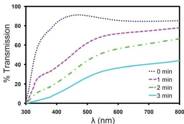
**Fig. 7** Light transmission through an ITO film subjected to electrophoretic conditions. The percent transmittance of light through an ITO-based electrophoretic device is plotted as a function of total exposure time to electrophoretic conditions.
